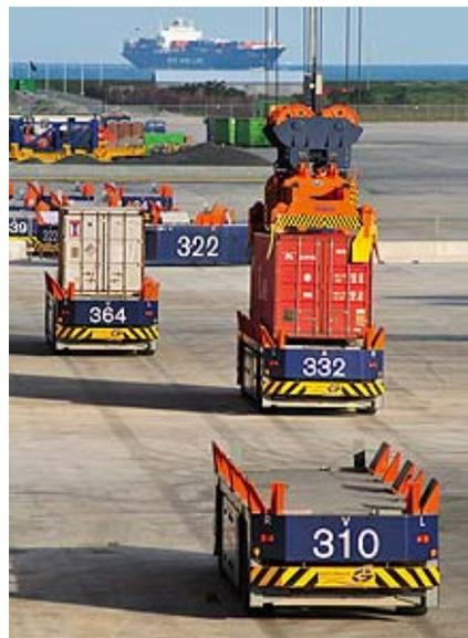
*Photo 6: Battery-electric drives for zero exhaust emissions
