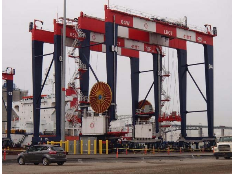
Photo 1: ASC (End-Loaded) with Medium-voltage cable reel
