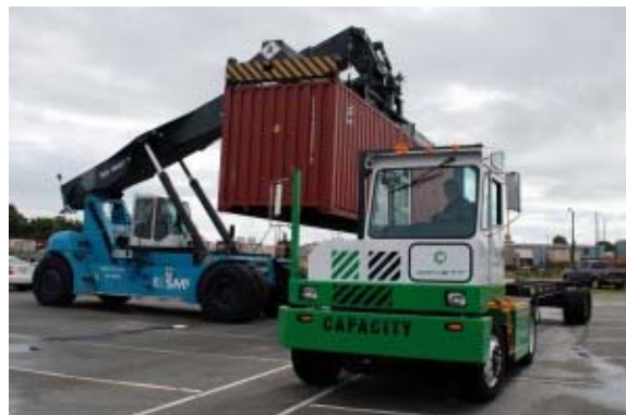
Photo 5: Electric hostler being test at Port of Los Angeles
