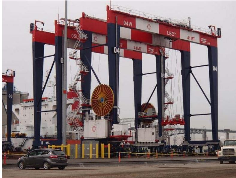
*Photo 1: ASC (End-Loaded) with Medium-voltage cable reel*
