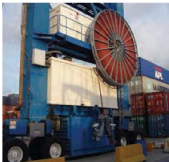
*Photo 4: E-RTG (Plug-in) with cable reel*
