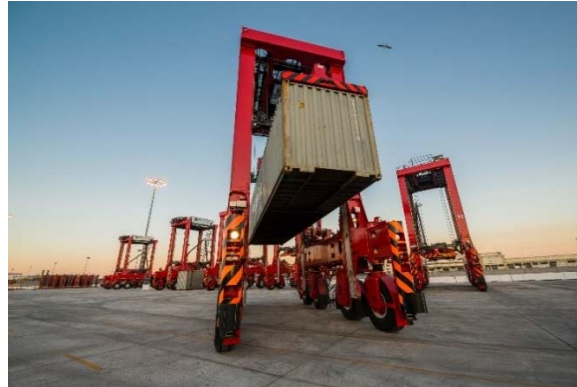
Photo 6: Automated Diesel Electric Straddle Carriers in Use at TraPac Terminal at Port of Los Angeles
