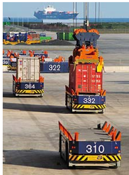
Photo 6: Battery-electric drives for zero exhaust emissions in the terminal AGV fleet in the Port of Rotterdam, Netherlands
