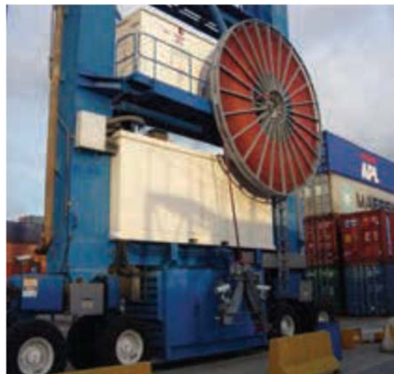
Photo 4: E-RTG (Plug-in) with cable reel
