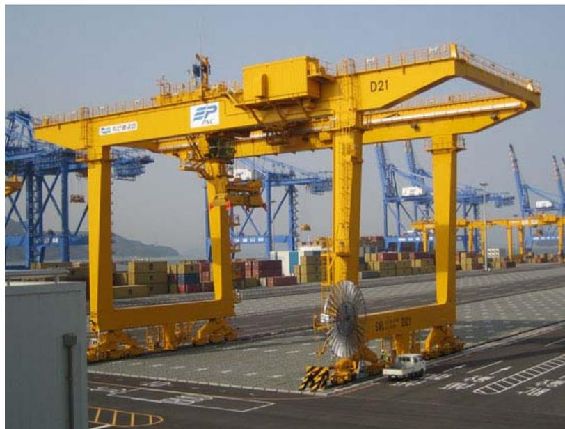
*Photo 2: RMG (side-loaded) with Medium-voltage cable reel*
